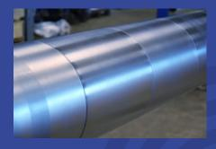
Hard chromium plated stainless spreader rolls enable easier and less expensive maintenance – there's no need to replace rubber sleeves during overhaul.
