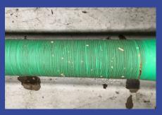
A rubber sleeve wears out unevenly during operation which leads to a non-uniform spreading effect on the web.
