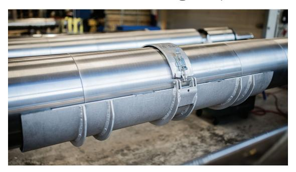
With Finbow lifting tray you can safely lift your spreader roll from the segments. Roll weight is distributed evenly between safe loading points and bearing alignment is not disturbed during lifting. With the help of the tray you can install rolls to the most demanding positions minimising the risk of a failure.
