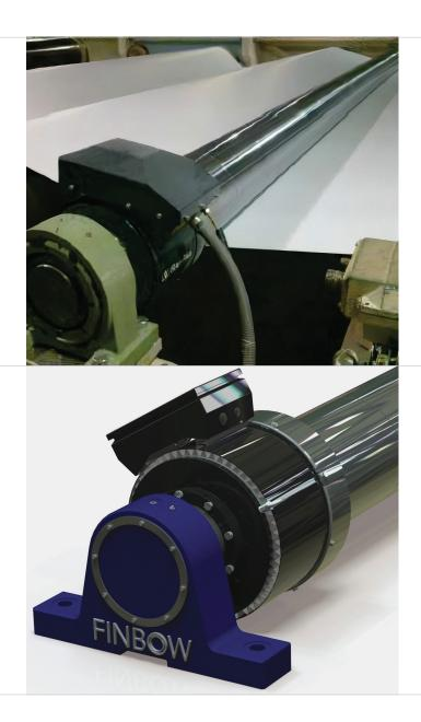
Delivery of the direct drive spreader roll for the dryer after online coating station
