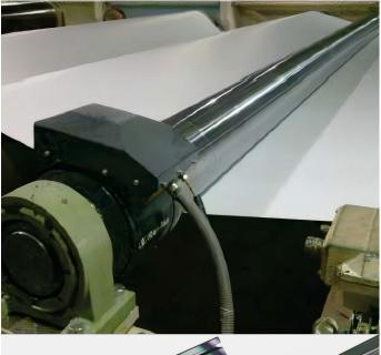
Delivery of the direct drive spreader roll for the dryer after online coating station
